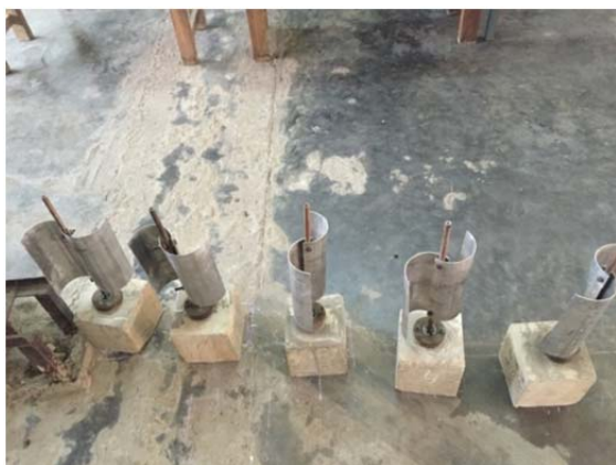
Fig. 1: When the wind turbine models are kept in an inclined manner to the direction of wind flow coming from the blower.
