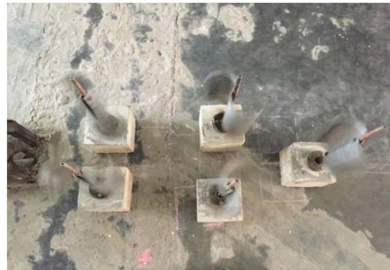
Fig. 2: When the wind turbine models are kept along the periphery of a circle in front of blower.
